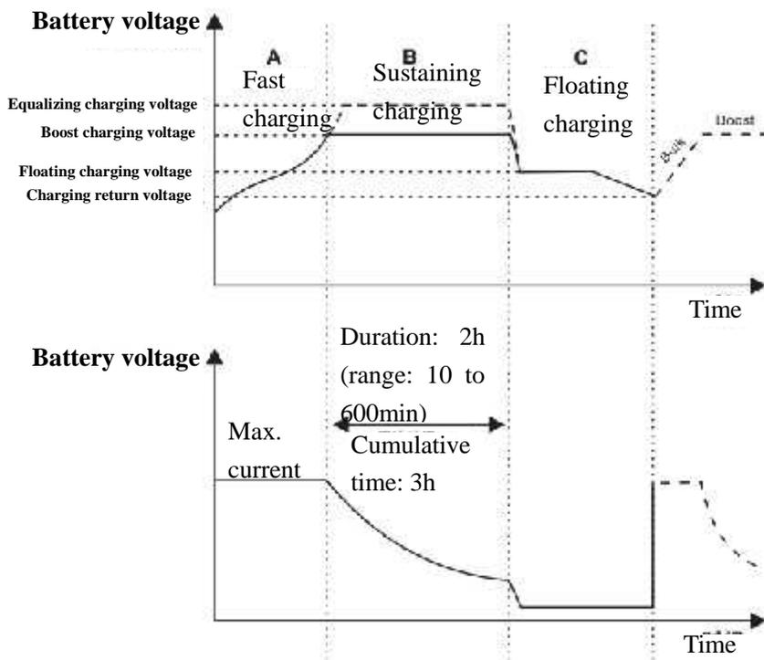
**Fig. 1-5 Battery charging stages diagram**
