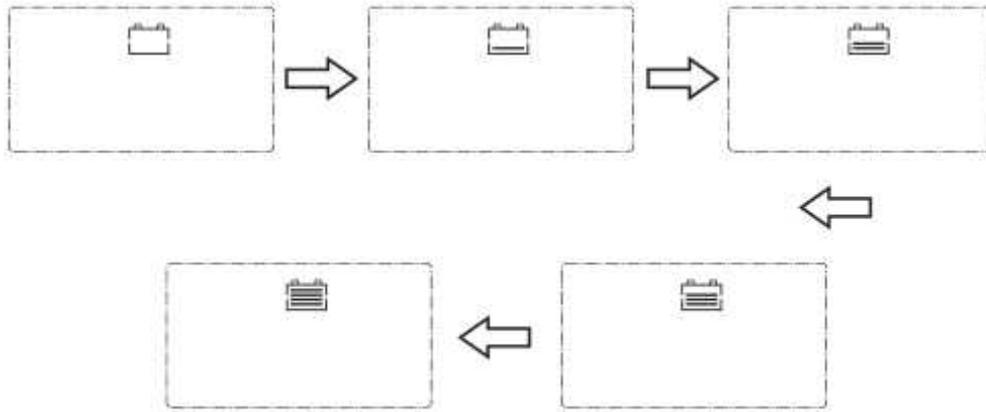
During startup, the 4 indicators will first flash successively, and after self-inspection, the LCD screen starts and displays the battery's voltage level which will be either a fixed voltage selected by the user or a voltage automatically recognized.
